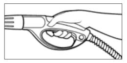
Step 5 Plug the power cord into the power outlet. Trigger the gun to eliminate trapped air, wait for a steady flow of water to emerge from the spray nozzle.
